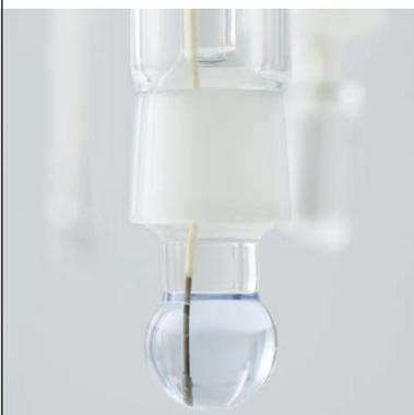
Thanks to the ARGENTHAL™ reference system most METTLER TOLEDO pH sensors are filled with 3 mol/L KCl electrolyte solution. There is no longer a risk of contaminating your samples with silver ions. For measurements in non-aqueous samples or samples with low ionic strength a special bridge electrolyte is needed. Always make sure that your sensor is completely filled with clean electrolyte solution.
