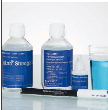
Whenever rinsing with deionized water is not sufficient, a special cleaning solution can be used to remove sample residues. Depending on the contamination, Pepsin-HCl or Thiourea is recommended. The InLab® storage solution provides optimal conditions for sensors during the time between measurements, be it short- or long-term storage. Find more helpful maintenance tips on [www.electrodes.net](http://www.electrodes.net)
