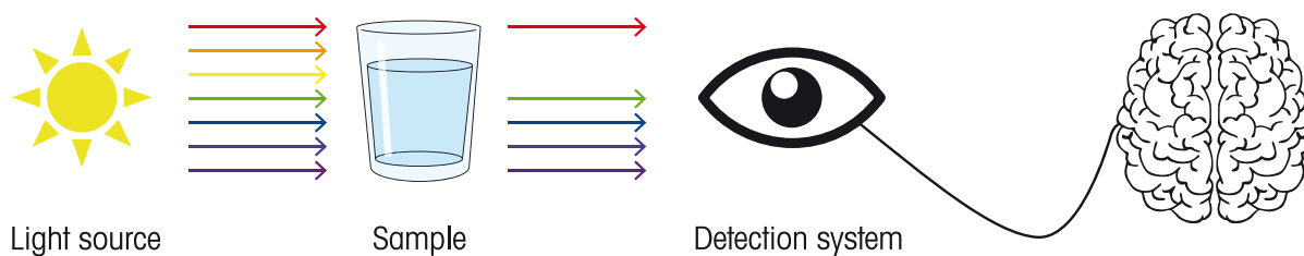
Figure 4: Light passing through a sample solution is partially absorbed by the components.
