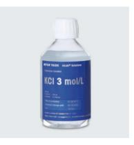
Thanks to the ARGENTHAL™ reference system most METTLER TOLEDO pH sensors are filled with 3 mol/L KCl electrolyte solution. There is no longer a risk of contaminating your samples with silver ions. For measurements in non-aqueous samples or samples with low ionic strength a special bridge electrolyte is needed. Always make sure that your sensor is completely filled with clean electrolyte solution.
