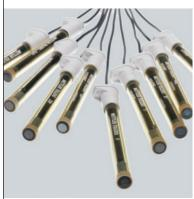
It is important to fill the reference electrode of every ISE with the recommended electrolyte solution. The correct electrolyte will minimize junction potentials and provide optimum temperature and response time. The electrolyte must be refilled or replaced regularly in order to maintain good electrode performance. For more information please refer to the electrode manual.
