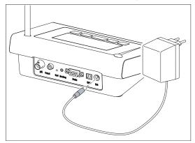
3 Plug the AC adapter into the wall socket.
