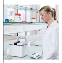
FastTrack UV/VIS technology guarantees that the instrument is ready at all times. No warm up time is needed for the Xenon flash lamp to reach stability, which speeds up measuring time. As the lamp is only used for real measurements, its lifetime is greatly increased.
