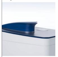
LockPath enables the measurement of wide concentration ranges from 6 to 15,000 ng/µL of dsDNA without further dilutions within 2 seconds per pathlength. The most suitable pathlength can be automatically locked. The arm design prevents the sample from drying out during measurement, significantly increasing repeatability.
