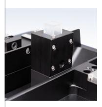
FastTrack UV/VIS technology comprises modern fiber optics in combination with array detection and a Xenon flash lamp. A full spectrum scan is performed within just 1 second. Stable lamp intensity conditions significantly increase throughput, as multiple reference measurements are not needed during sample series.
