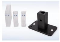
Cuvettes: 1 cm, 5 cm pathlength optical and quartz glass, 700 µL micro cell quartz glass, 440 µL flow cell quartz glass. Holders: 1 cm, long pathlength, solid sample, tube.
