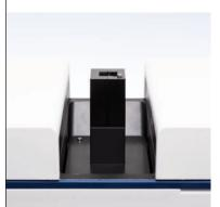
Thanks to the FastTrack UV/VIS technology, there are no moving parts in the instrument, and thus it reduces the risk of misalignment. This not only contributes to accuracy, not also brings a low requirement of maintenance.
