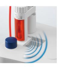
Is the correct titrant installed? Is the concentration right? Has the concentration determination expired? All this information is stored on the burette chip and the titrator automatically verifies all parameters when a titration is started. Errors occurring during the installation of resources are now a thing of the past. Be assured with the Plug & Play feature, safe titration could not get any simpler.
