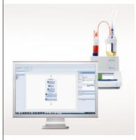
METTLER TOLEDO Titrators offer a broad range of possibilities to handle your data. Choose whether to export as CSV, PDF or XML files. Devices such as printers or memory sticks can be connected via the USB port and are automatically recognized. For full data security LabX<sup>®</sup> titration PC software supports the user in every action performed with the titrator. All results are stored in the LabX database.
