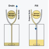
The reagents play an important role in the coulometric Karl Fischer titration. The Reagent Control keeps an eye on the important parameters so that once the maximum capacity is reached the user is prompted to replace the reagents. Contact with any of the reagents is avoided and the user always has an optimal system, ready to use and prepared to generate correct, repeatable results.
