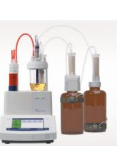
Contact with Karl Fischer reagents should always be avoided. The Solvent Manager takes care of filling, draining and exchange of the reagents. It is fully controlled by the titrator which offers One Click access to all tasks. LevelSens additionally increases security by monitoring solution and preventing overflow in the waste bottle.
