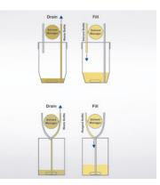
The solvent needs to be replaced regularly in order to guarantee consistently correct results. The Solvent Control supports the user by monitoring different parameters. Even when an instrument is running on Standby the Solvent Control is active and automatically starts conditioning of the fresh solvent after exchange. With minor user interaction the system is always kept in optimum condition ready to ensure a quick, accurate result whenever required.
