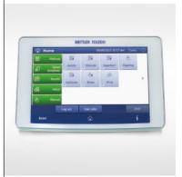
The Titration Excellence line ensures you get your results easily and quickly. The Shortcuts, which can be set up specifically for each user, are extremely helpful. Whether you want to calibrate electrodes, rinse burettes or start methods — you can define a Shortcut for any operation you like and store it on your Homescreen.
