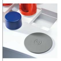
A SmartSample reader is installed as standard on all Excellence instruments. Wireless data transfer from balance to titrator is now possible on single samples, eliminating transcription errors due to manual entry. The Smart-Sample solution is therefore an intelligent choice for both single-and automated multi-sample titration.
