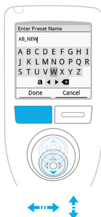
Under "Enter Preset Name," use the joystick to move to letters and press the joystick in to select them. Joystick to the left side of the bottom row of buttons to access lowercase letters and numbers. Joystick to the right side of the bottom row of buttons to delete a character. When the preset name is complete, press the left button – **Done**.
