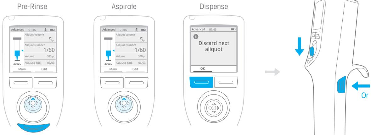
Press the left button, **Main**, and select **Manual**. Joystick up to aspirate a small volume. Then, push the Eject button below the joystick. NanoRep asks, "Empty tip?" Press the left button, **Continue**. The tip empties.
