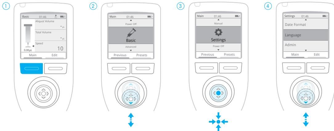
Press either blue button to power on NanoRep. A welcome screen displays, then shifts to the basic work screen. Press **Main**.
